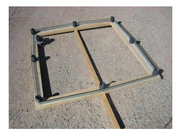
I built a square frame for this loop, 24 inches on a side, again out of 1 x 2 inch wood, commonly
